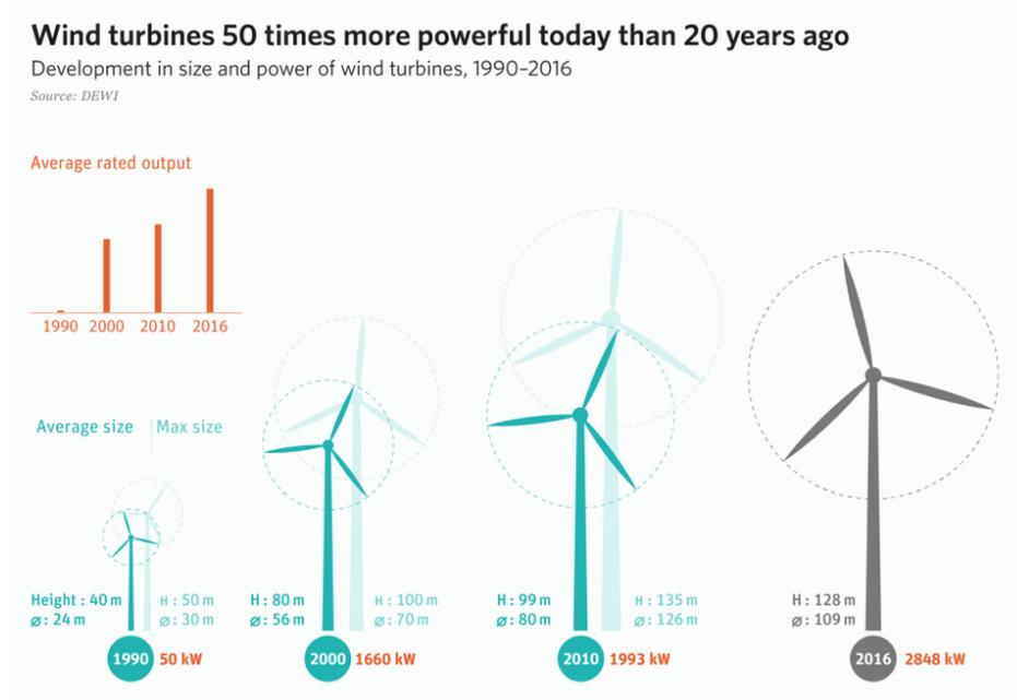
Development in Size and Power of Wind Turbines from 1990 to 2016 [3]
